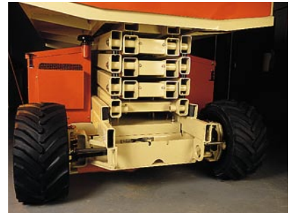
Strengthened Arm Stack for Improved Stack Rigidity
